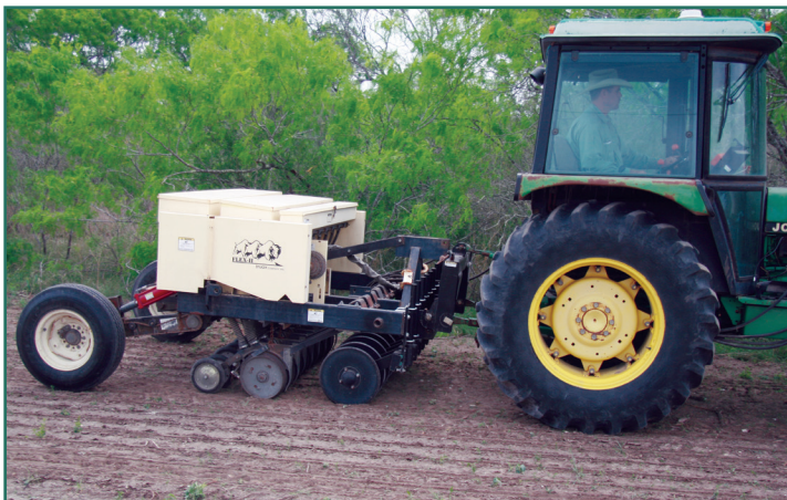
Figure 3. A seed drill specifically designed to handle native seeds.
